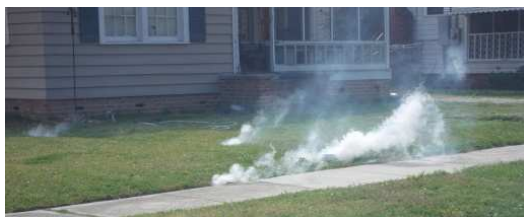
Smoke emerging from a defective sewer lateral beneath a lawn.
