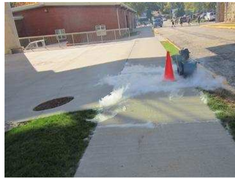
Smoke is pushed into the system and emerges from cracks in the sidewalk
