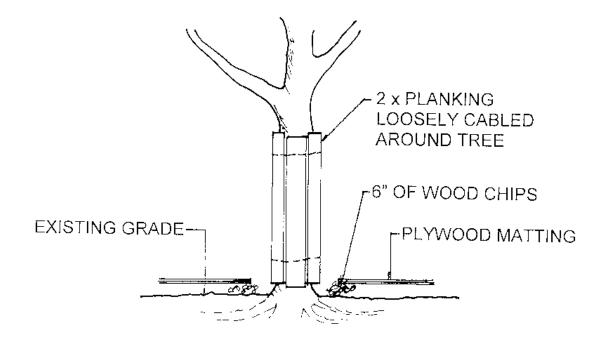
Note: This protection is to be used when circumstances do not allow Typical Tree Protection (see detail, page 11). Install 6" of wood chips and use plywood matting over wood chips in areas where equipment must operate Protect trunk with planking to reduce scarring by equipment. Remove planking, matting and mulch as soon as operations are finished.
