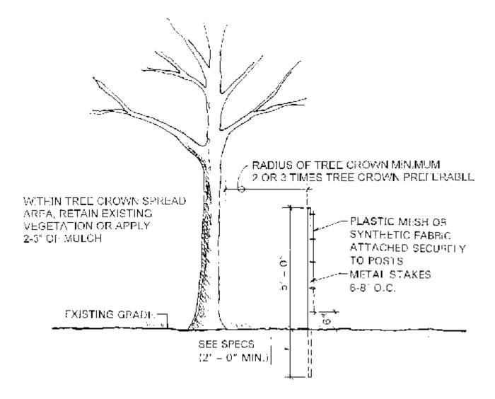
Note: This barrier is intended to keep construction equipment, personnel and materials from compacting the soil around tree roots and damaging the trunk or limps of the tree.
